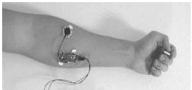
Figure 5. Placement of surface electrodes on the arm (The figure is taken from [23]).
